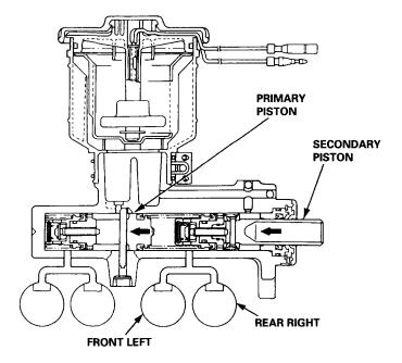
(2) In case of leaking from the secondary system
