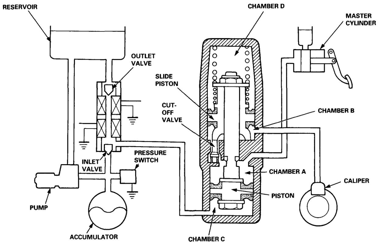
If brake inputs (force exerted on brake pedal) are excessively large and a possibility of wheel locking occurs, the control unit operates the solenoid valve, closing the outlet valve and opening the inlet valve. As a result, the high pressure is directed into chamber C, the piston is pushed upward, causing the slide piston to move upward and the cut-off valve to close.
